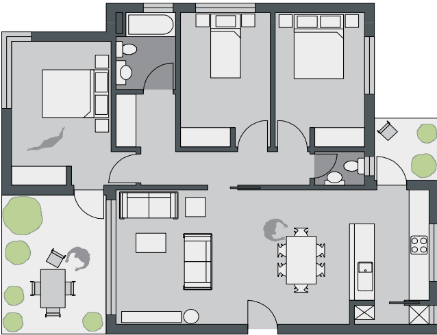
Figure 4E.4 Building layout should maximise balcony use by allowing access from the main living area and a bedroom (where possible). Secondary balconies provide further amenity to apartment living and are best accessed off kitchens and laundries
