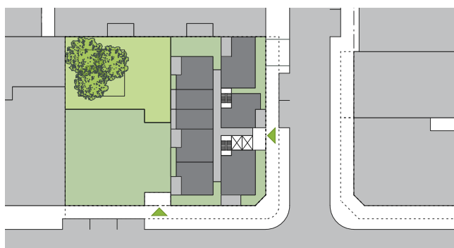
Figure 4F.2 The total number of apartments accessed off one circulation core should be eight or fewer
