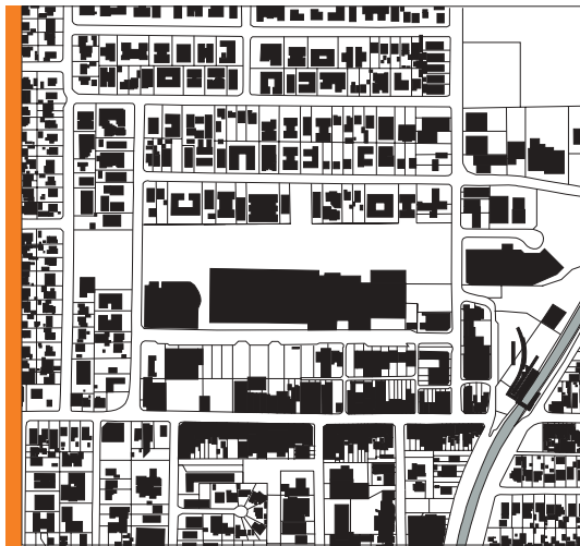
01.01. A figure ground drawing illustrates the relationship between building to open space and can help to identify different building types (houses, courtyard apartments, shopping centres, main street shops).
