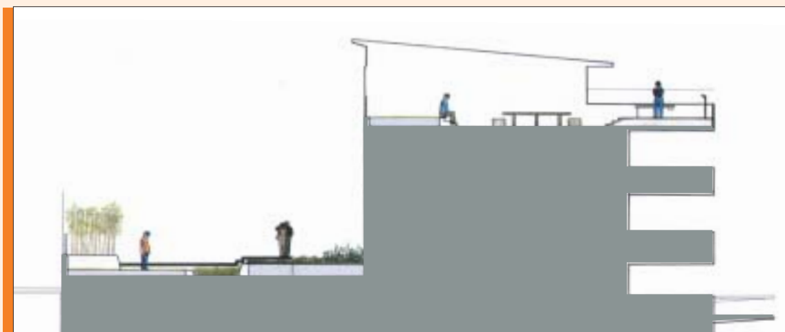
02.33. This section illustrates the suitability of the landscape design to limited soil depths on a roof structure.
