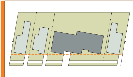
01.66. Street setbacks can be defined with a minimum setback and a facade angle in areas where angled lots exists and a response to the existing street pattern is desired.
