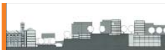
A4.07. A generally consistent height for new residential development in Pymont follows the line of the ridge, with a sharp change in level accentuating the existing cliff edge.
