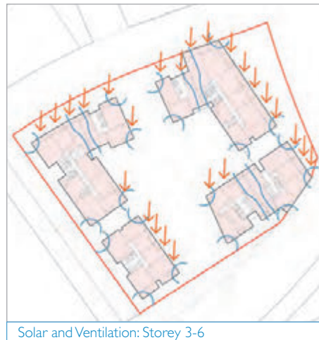
Solar and Ventilation: Storey 3-6
