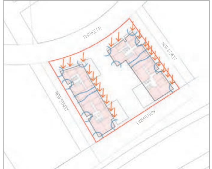
Solar and Ventilation: Storey 7-8
