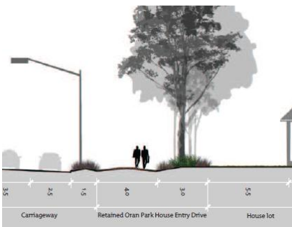
Potential design for walking and bicycle paths along Dawson-Damer Drive. (Source: Aecom Landscape and Visual Analysis)
