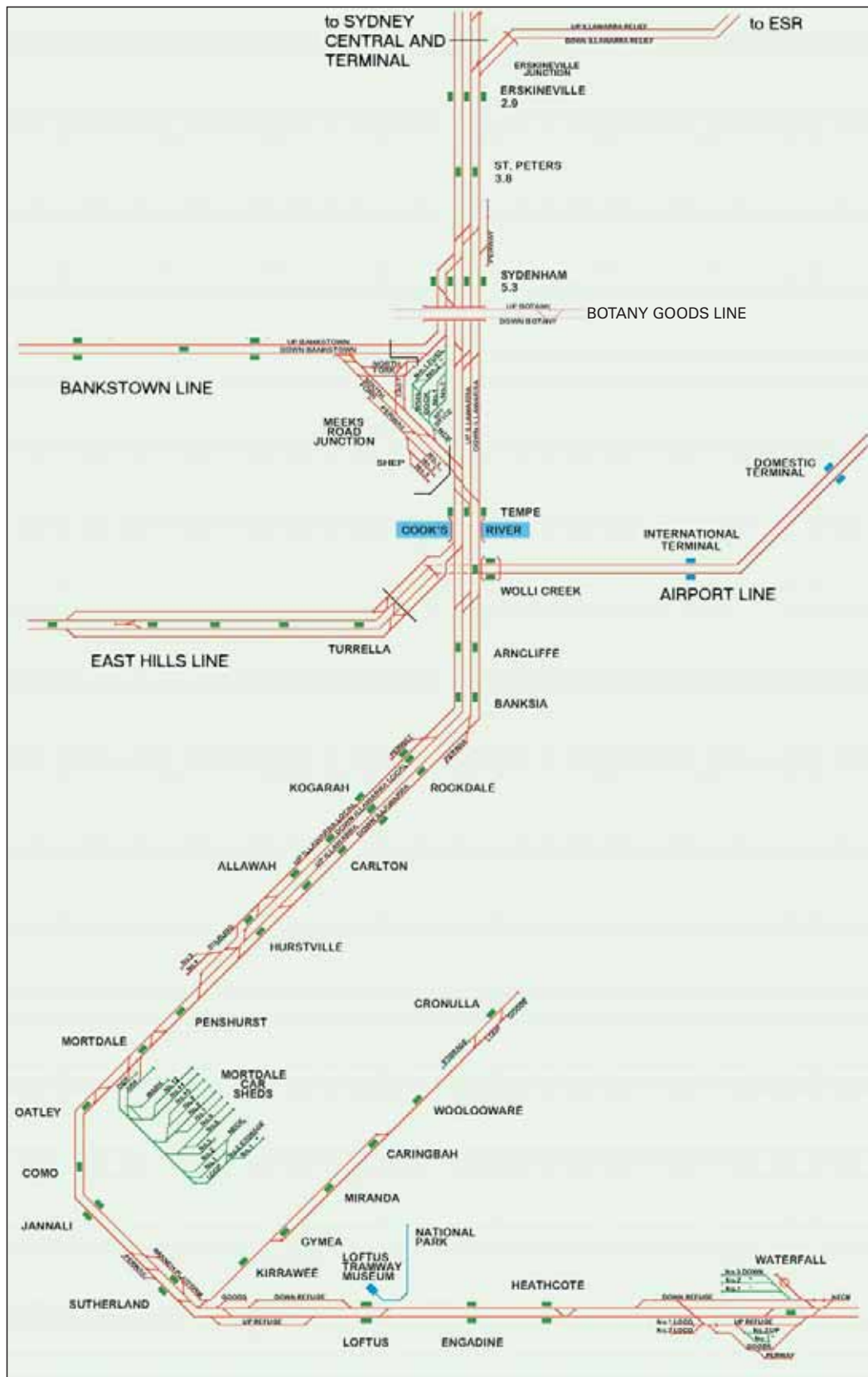
Figure 4.1 DIAGRAMMATIC LAYOUT OF HEAVY RAIL LINE BETWEEN SYDENHAM AND WATERFALL
