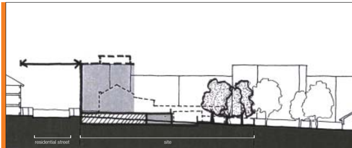
02.09. North South Section. A street edge alignment is proposed to help define the streetscape. The carpark, located under the building footprint, allows for deep soil planting in the rear garden. The topography falls away from the building exposing the carpark along the rear garden. There is a potential for garden apartments to locate along this edge and to provide an improved elevation to the communal open space.
