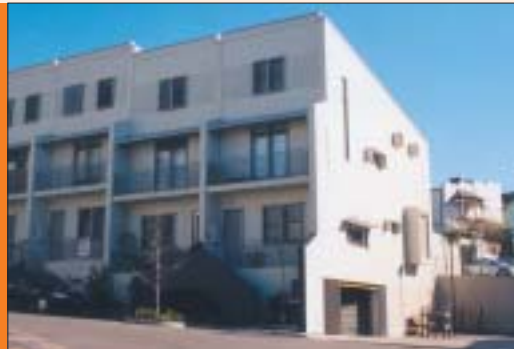
02.52. The location of the carpark entry on the secondary facade minimises its impact on the primary streetscape.
