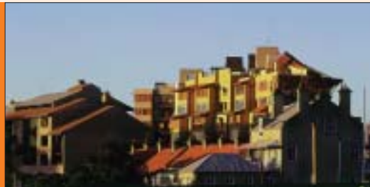
03.52. This roofscape design subdivides the appearance of a large building into multiple volumes sympathetic to the existing neighbourhood.
