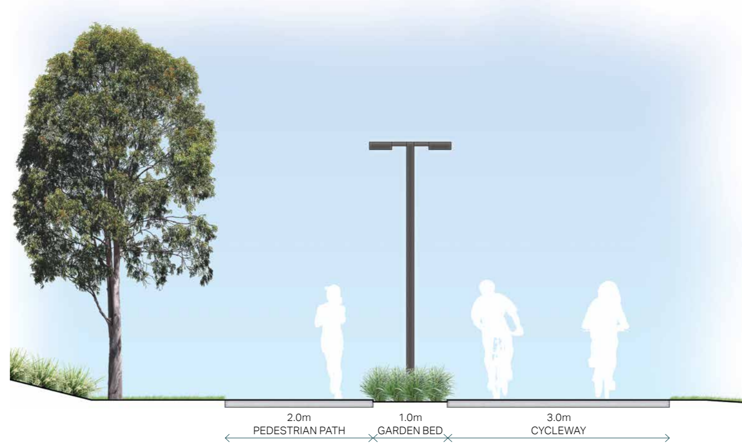
DETAIL AREA: PARRAMATTA VALLEY SEPARATED CYCLEWAY 1:50@A3
