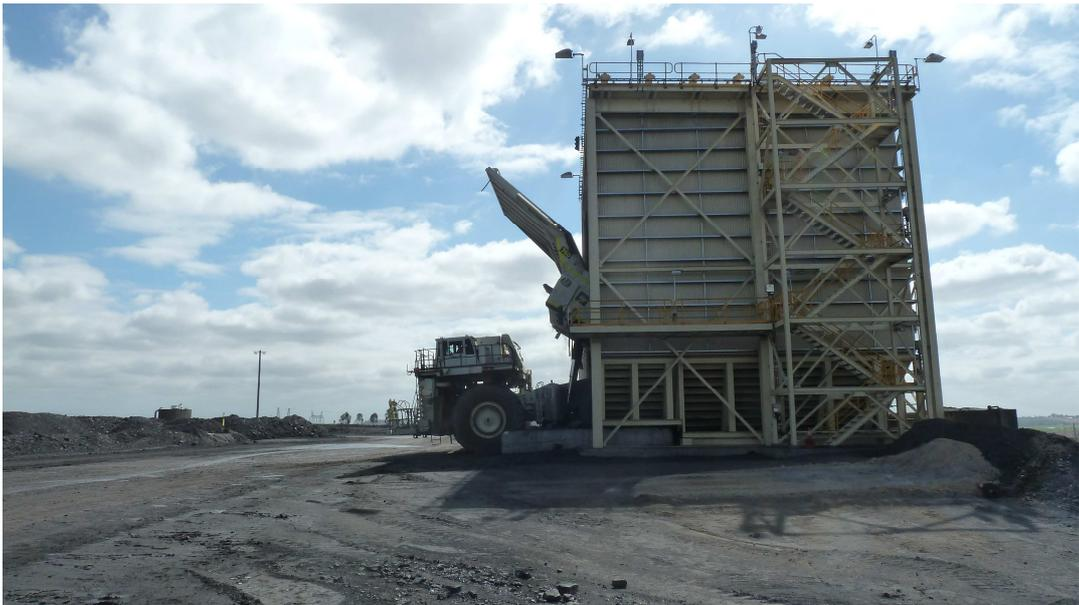
**A truck unloading coal in the new coal hopper hood at the Mt Thorley Warkworth mine.**
