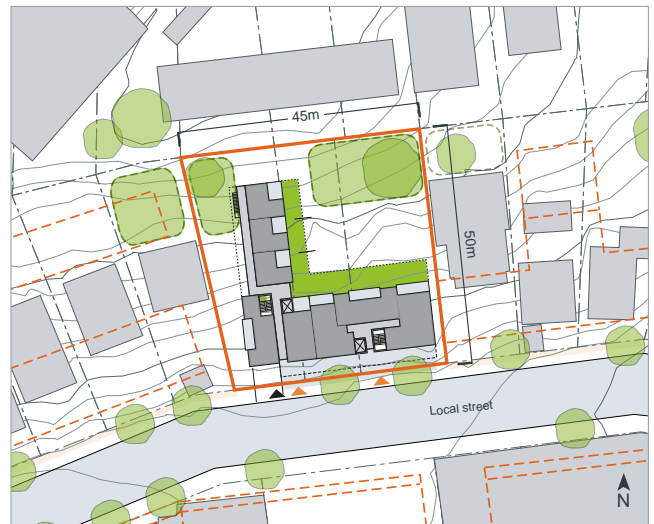
Figure 1B.7 The site scale is a detailed analysis of the development's immediate context and should include the site itself, the street it addresses and surrounding properties. All proposals should address this scale
