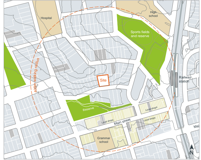
Figure 1B.5 The neighbourhood scale outlines the urban grid and block structure including streets and open spaces, significant topography, heritage and civic and community uses. Proposals for individual or small groups of apartment building sites should address this scale
