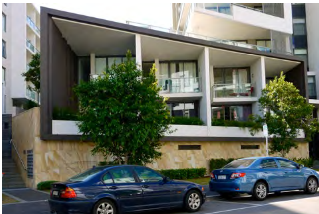
Figure 4E.11 Setting the balustrade back from the building edge allows for landscaping towards the street for increased privacy
