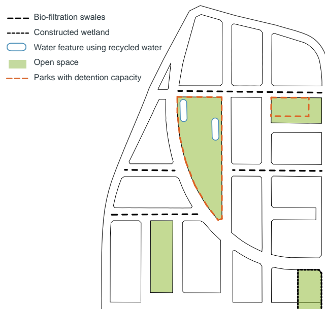
Figure 4V.1 Streets and parks of larger developments should be designed to treat stormwater runoff and accommodate flooding events
