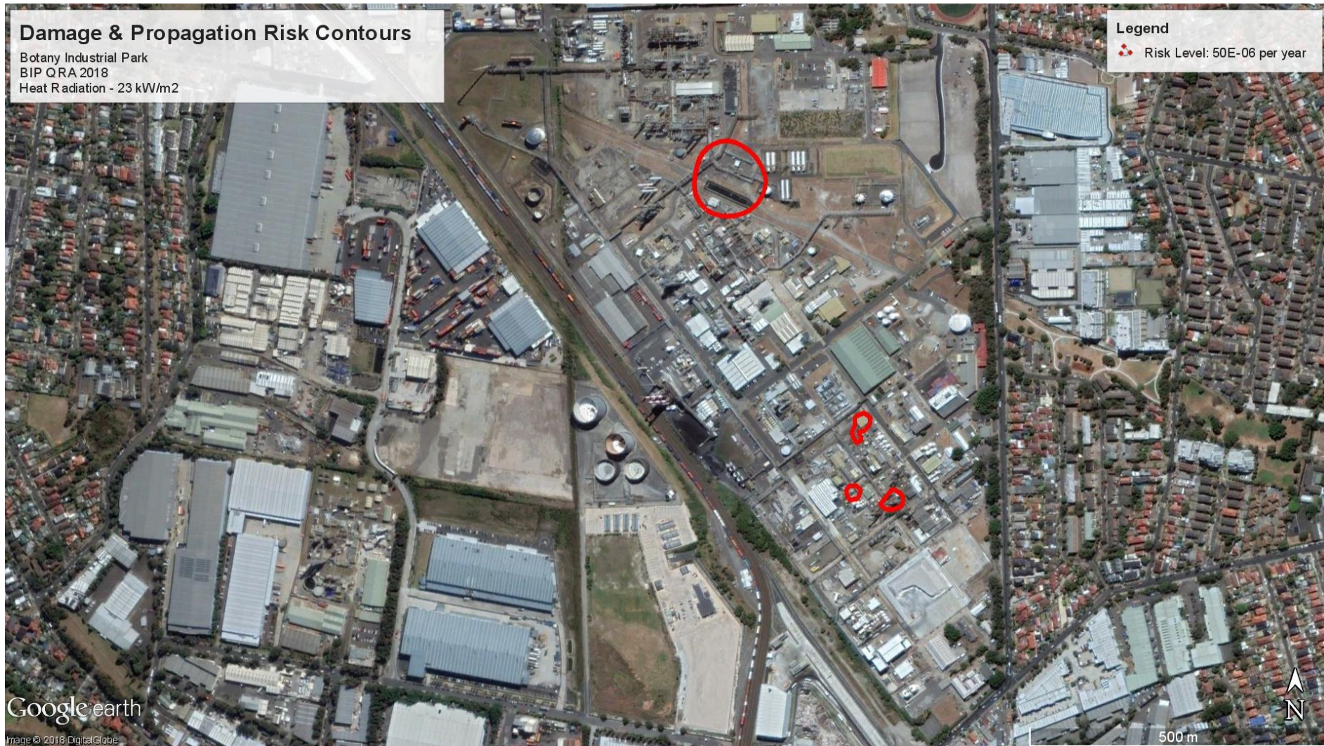
FIGURE 9.6: CUMULATIVE ESCALATION RISK, HEAT RADIATION EXCEEDING 23 KW/M 2 BIP
