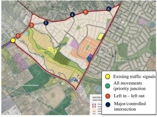
Figure 21 Planned intersections on sub-arterial
