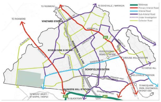
Figure 18 Road hierarchy and rail crossing alignments
