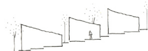
Modules on greater than 10° slope
