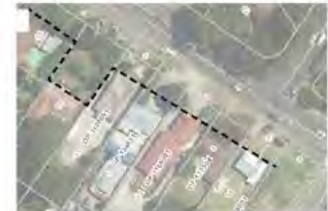
INCONSISTENT SETBACK IN STREETSCAPE Creating difficulties to comply with solar access
