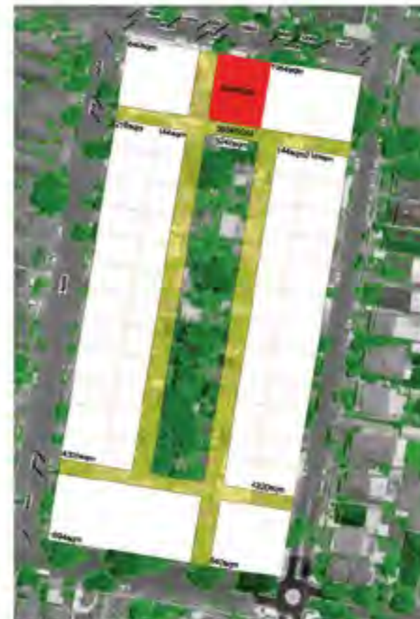
PROPOSED BLOCK - 2.09 Hectares 48 Terraced Dwellings on 8640 sqm 66 Apartments on 4438sqm @ 1:5:1 = 6657sqm developable area. 1 Public-Community Building on 630sqm 1 Public Park on 3240sqm 4 Streets on 3534sqm
