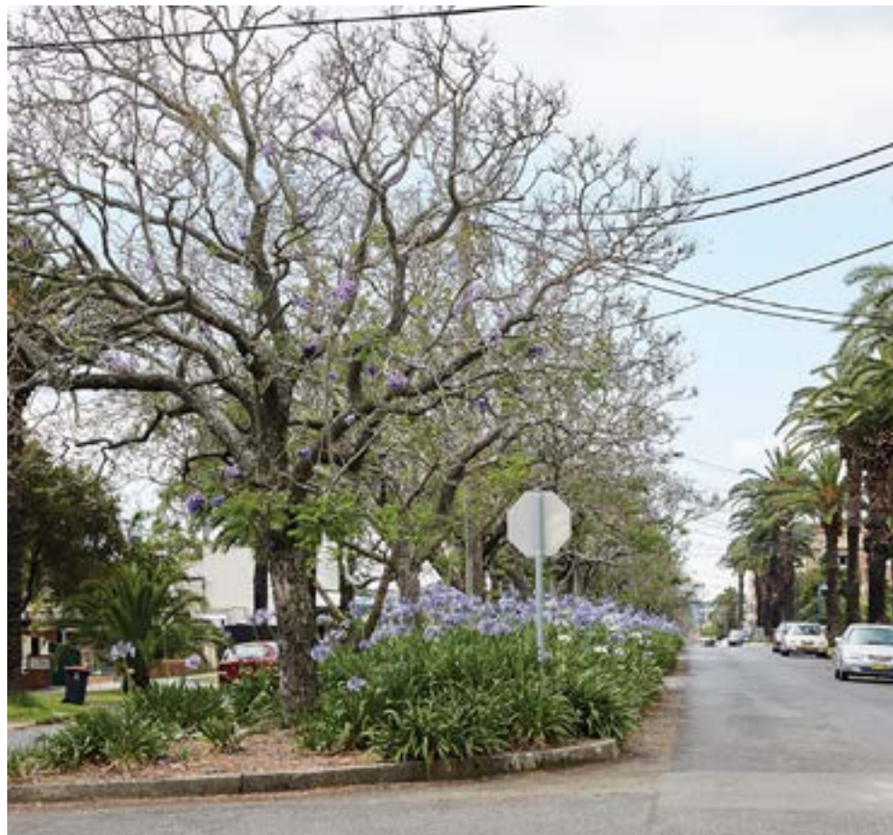
Figure 11: Raised kerb and understory planting along the street – provides good separation of vehicles and pedestrians
