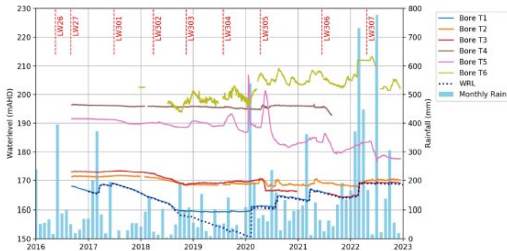
Figure 3 Groundwater hydrographs for bores T1 to T6 compared with reservoir water level and rainfall
