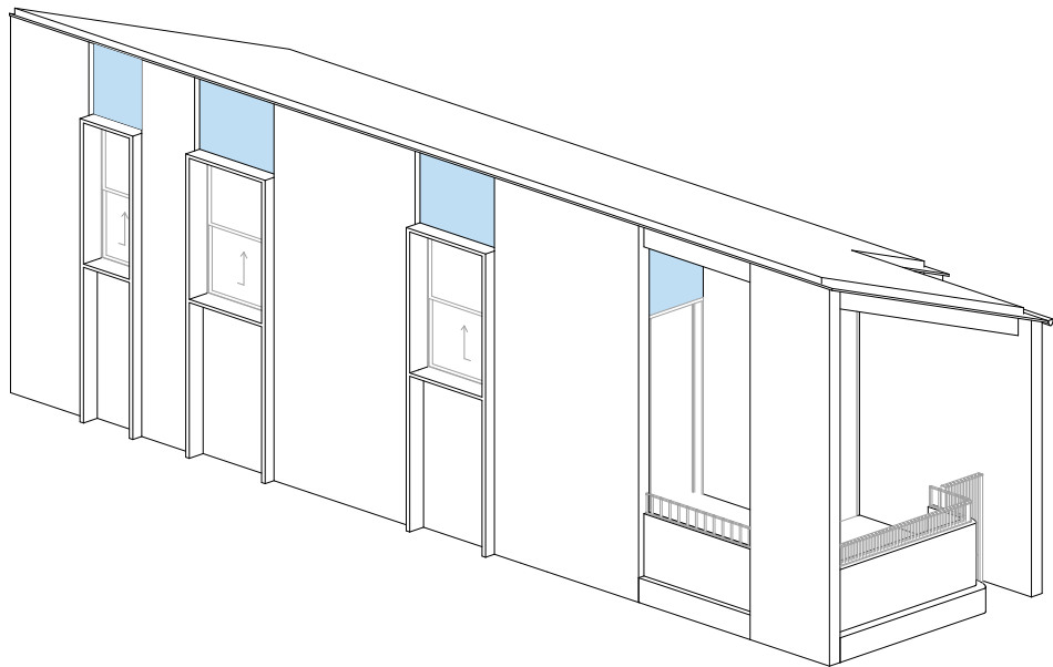
1 OPTION 1 REDUCTION OF GLAZING IF ORIENTATED SOUTH OR INCREASED THERMAL PERFORMANCE IN GLAZING
