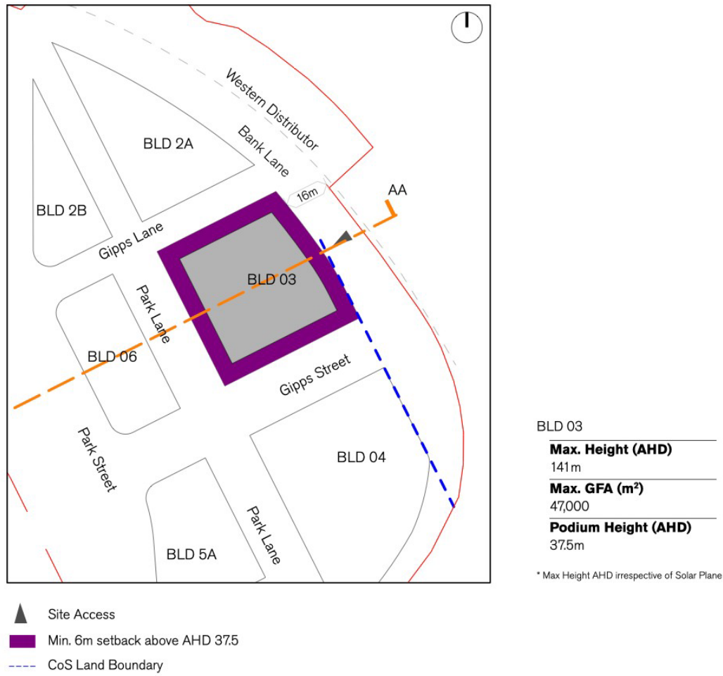
Figure 43 Block BLD 03 controls
