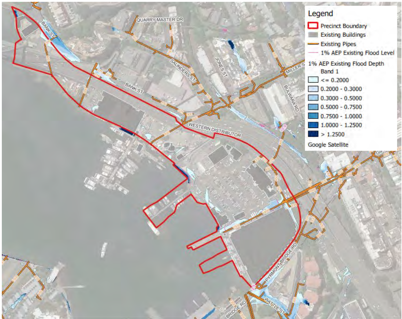
Figure 3-5: Existing 1% AEP Flood Depth
